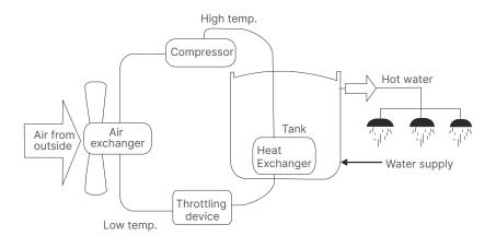
• Heat Pump collects environmental heat via collector systems and refrigerant is circulated which absorbs the heat, boils and evaporates.
